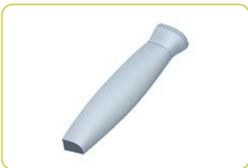
The finished handle of the scraper from Pro/ENGINEER. This image would precede the blade sketch image
