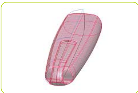
Analyzing the final surface model of the Flash Drive in Pro/ENGINEER
